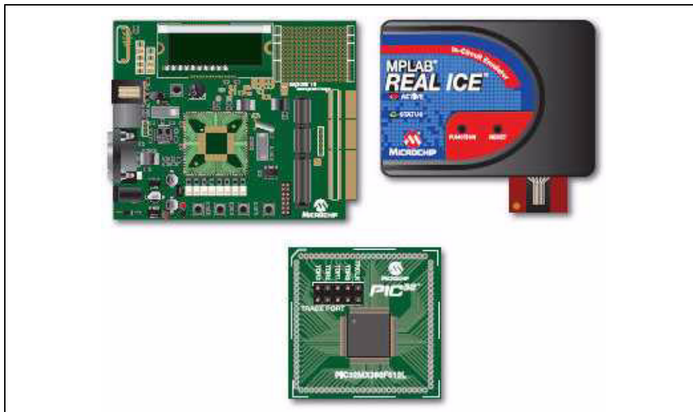
FIGURE 5-11: EXPLORER 16, MPLAB ® REAL ICE ™ AND PIC32MX360F512L PIM
